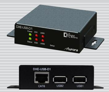
The DXE-USB is a single cable USB extender capable of transmitting bi-directional USB2.0 over a CAT 5e/6 cable. Together (DXE-USB-S1) the DXE-USB-H1 (Host PC Side) & DXE-USB-D1 (Device Accessory Side) work together to extend to USB up to 220 feet at a full 480Mbps.
