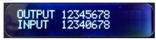
The LCD will reflect what Output is routed to which input when in an idle state. The ASP-442A (4x4) will only show 1,2,3, & 4 on the LCD unlike the ASP-882A which will show 1-8 since it is an 8x8.
